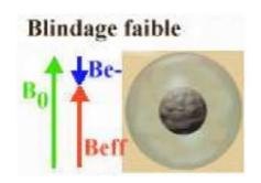
$$\nu_i = \frac{\gamma}{2\pi} B_{eff} = (1 - \sigma_i) \frac{\gamma}{2\pi} B_0$$
